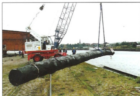
Mastrohling am Kran
